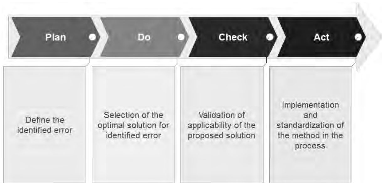
Figure 3. Implementing the PDCA cycle in the developing process of a poka yoke mechanism. Source: Own processing
