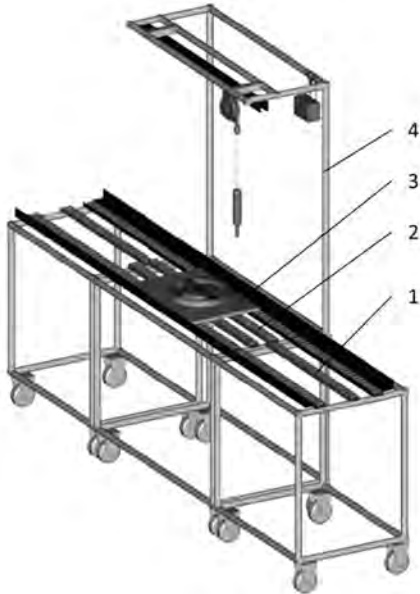
Fig. 7. Design of transfer system linking the workstations
