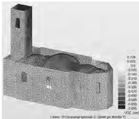
Displacements in direction z
