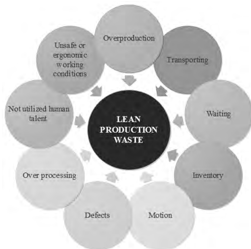
Figure 1. The 9 losses identified in a production process. Source: Own processing based on information from Taiichi 1998 and Magdalena and Beata, 2017
