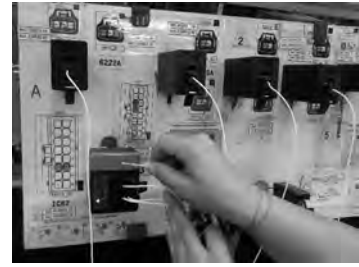
3.c. Touch the terminal on the metal side and it illuminates the cell
