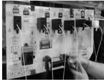
3.b. Terminal insertion into top and bottom connectors crossing wires through bellows
