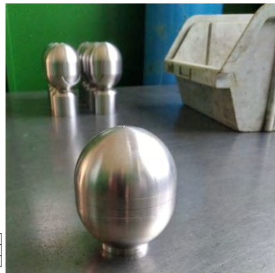
Figure 6. Body of the nozzle system without machined slots
