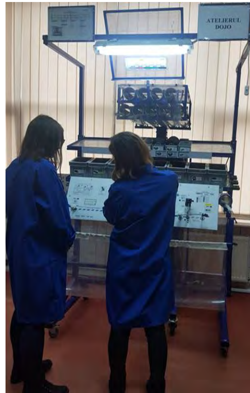
Figure 17. DOJO workstation for wiring assembly
