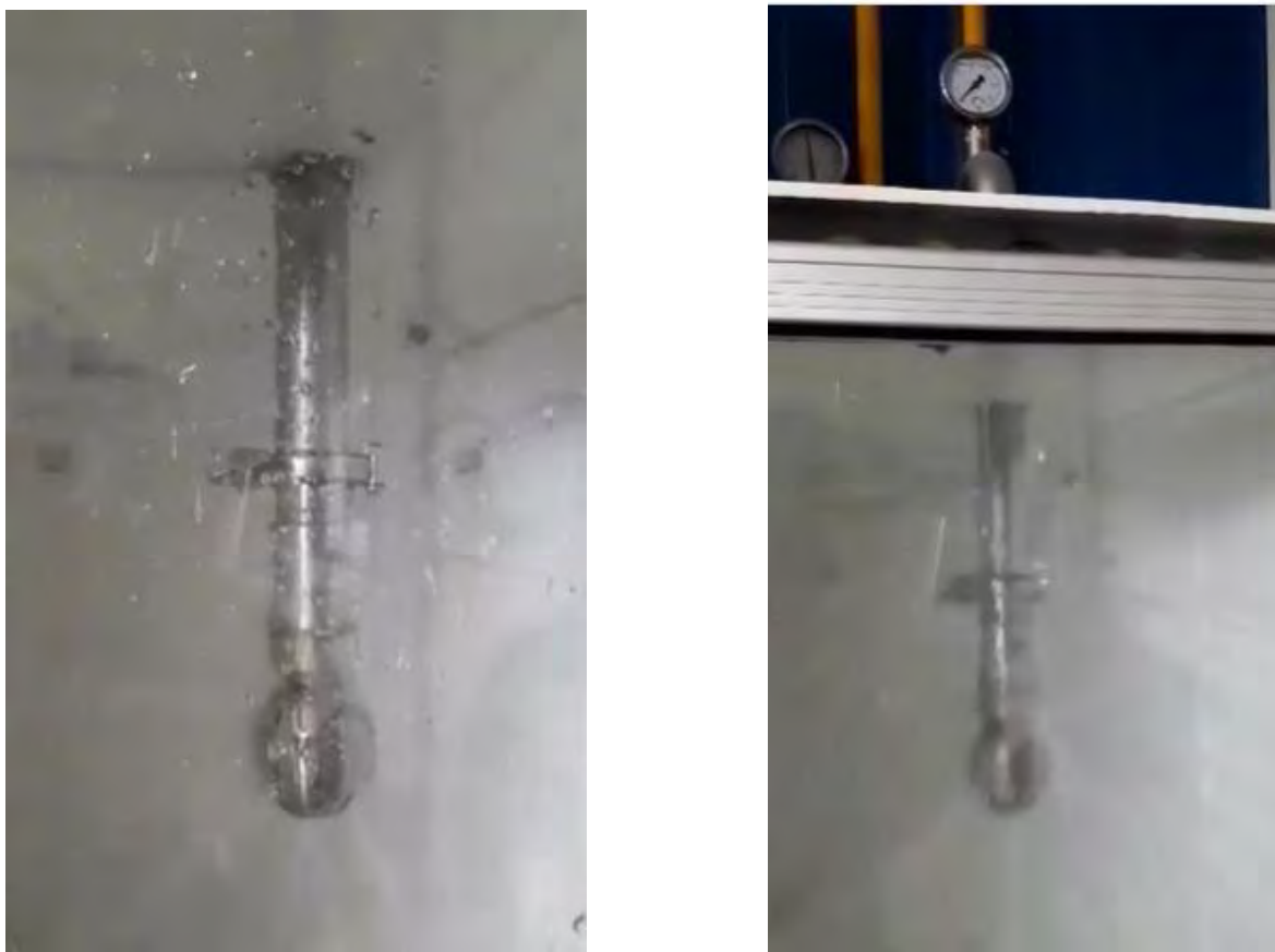
Figure 8 - Images from the 360° spray head test
