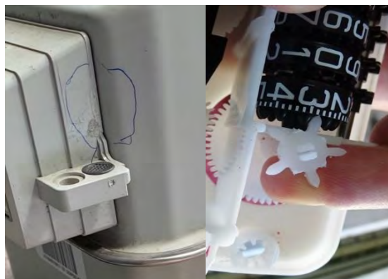
Figure 2. Intervention on the integrator and cutting the gear teeth of the mechanical index
